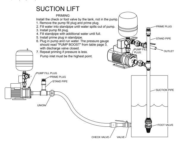
The pump inlet must also be the highest point. There can be no humps in the line as shown here:
