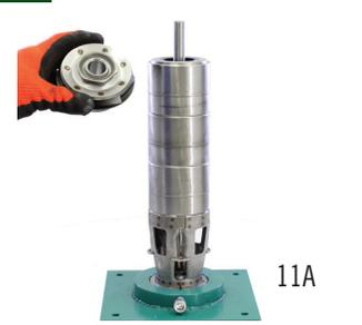
Use WRENCH FOR IMPELLER NUT to tighten (clockwise)
