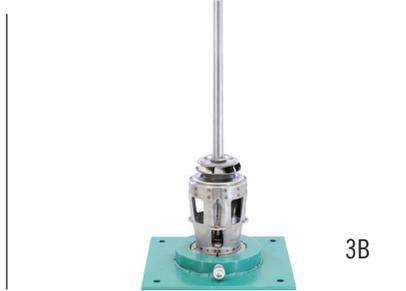
**4** Use WRENCH FOR IMPELLER NUT to tighten (clockwise)
