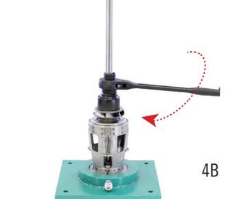
**5** Place TORQUE TESTING NUT and use TORQUE WRENCH with INSERT to tight at correct torque (clockwise)
