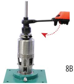
Use TORQUE TESTING NUT and WRENCH to tight at correct torque (clockwise) (STEP 5)
