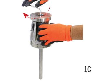
**2** Set down on FIXTURE SEAT and tighten using HEXAGONAL ALLEN TOOL (clockwise)
