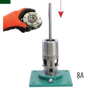
Use WRENCH FOR IMPELLER NUT to tighten (clockwise)
