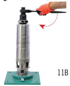
Use TORQUE TESTING NUT and WRENCH to tight at correct torque (clockwise) (Step 5)
