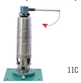
**12** Loosen with Allen Tool, remove from Fixture Seat. Remove 4" Jig with Allen Tool from Assembly
